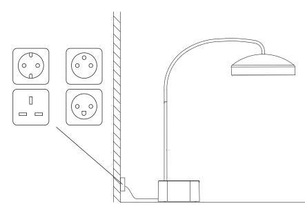
NOTE: The DISC will be delivered with a supply cord of 6feet (1 m 90) bold wall plug.
