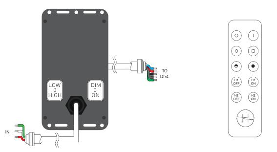
To connect the DISC to the main power, a 2-pole, 3-wire grounding connection is required consisting of 2 hot wires (with an output of 220-240V AC 60 Hz) and 1 grounding wire in a size not less than 1.5  $\text{mm}^2$  / 16 AWG. For safety reasons 2.5  $\text{mm}^2$  / 14 AWG is recommended.
