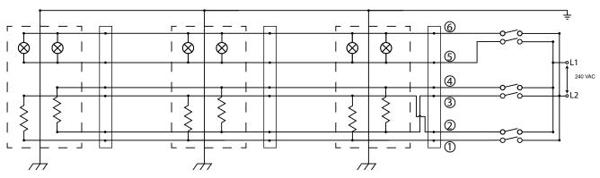
To connect the BEEM to the main power, a three pole connection is required consisting of two hot wires (with an output of 110-120/220-240V AC-60 Hz) a Neutral wire and one grounding wire in a size not less than  $1.5 \text{ mm}^2 / 16 \text{ AWG}$ . For safety reasons  $2.5 \text{ mm}^2 / 14 \text{ AWG}$  is recommended.
