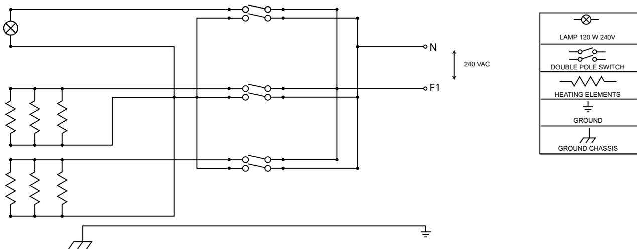
**To connect the DOME to the main power, a 3 pole connection is required consisting of 2 hot wires (with an output of 220-240V AC 60 Hz) and 1 grounding wire in a size not less than 1.5 mm<sup>2</sup> / 16 AWG. For safety reasons 2.5 mm<sup>2</sup> / 14 AWG is recommended.**
