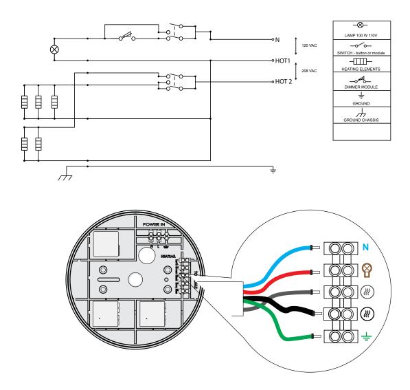
To connect the DOME to the main power, a three phase connection is required consisting of 3 hot wire and a nuetral (with an output of 120/208V AC - 60 Hz) and 1 grounding wire in a size not less than 2.5 mm<sup>2</sup> / 14 AWG.
