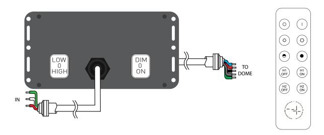
To connect the DOME to the main power, a single phase connection is required consisting of 2 hot wire and 1 grounding wire in a size not less than 2.5 mm<sup>2</sup> / 14 AWG.
