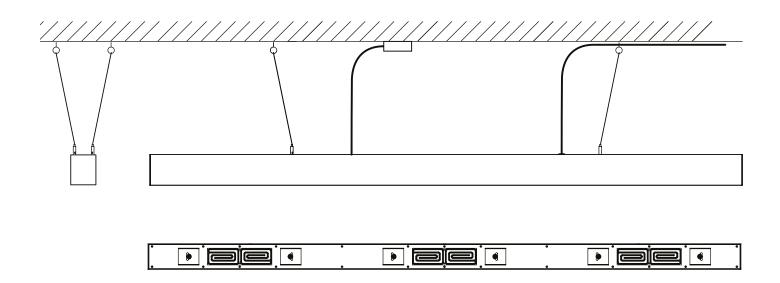
If the BEEM is installed in an area with windy conditions or with a high ceiling, it is adviced to hang the suspension cables slanted and angled to improve stability. Heatsail advices an angle of around 5° from the vertical axis to improve stability.
